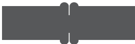
Crack On The Center Of Welding Bead, Not Enough Temperature or Long Change Over Time
